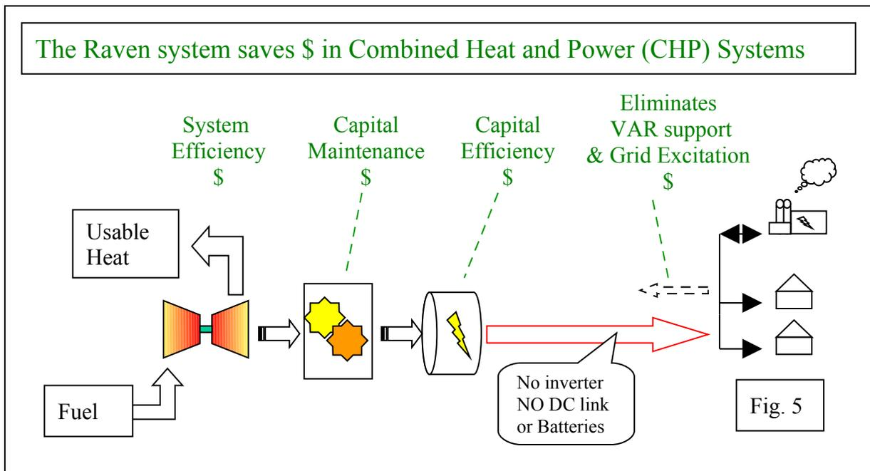
As described for other systems, Raven's variable speed generator technology can simplify or eliminate gearing and allow for system optimization at part load. Additionally, in co-generation plants the variable speed generator lets the system optimize efficiency while matching to the available thermal energy profile.
